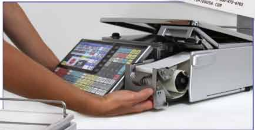
Quickly change Uni-7's label cassettes from the front, saving time for operators and customers alike.
